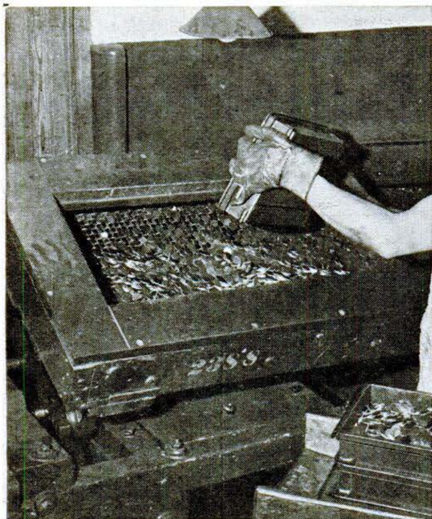
4. Here the output of the cutting machine is being dumped into a riddle, or large sieve. As it rocks back and forth any scraps of silver and broken or off-size blanks drop through the wire mesh into a salvage box. The metal, hardened from the rolling, next goes into an annealing furnace where it is softened by subjection to high temperatures. Cleaning comes next.
